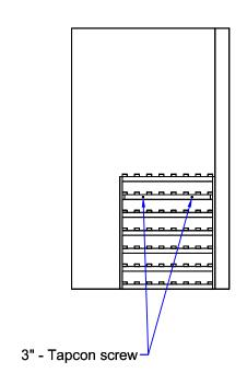
For uneven surfaces, like brick, we recommend using a slotted "L" bracket that you secure to the post with a 5/8" screw and then use a Tapcon screw to secure to the wall.
